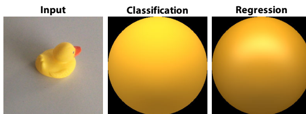
Figure 2. Regression often overestimates the shininess of objects. Therefore, we choose a classification-based approach.
