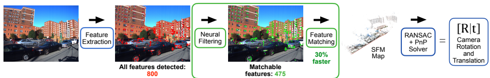
Figure 1: The proposed method augments a conventional pose estimation pipeline by adding a neural filtering stage that can filter out non-matchable features detected from a query image. The neural filtering stage can be easily plugged into existing pose estimation pipelines to efficiently select the most reliable features from all detected features . This reduces the number of features to be matched down to 30% on average (roughly 60% shown in the current example) for all datasets tested and improves feature matching times by increasing its speed while maintaining the final pose estimates.
