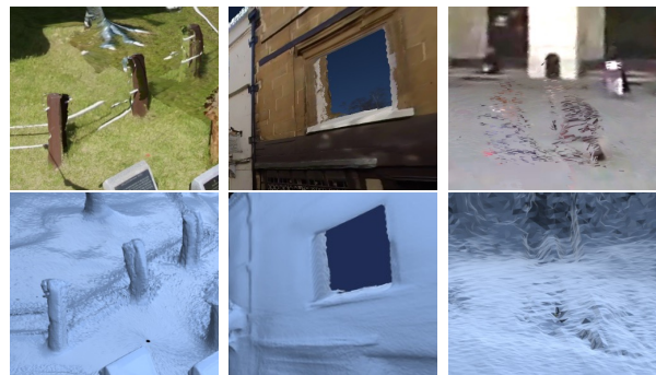
Fig. 12. Example failure cases. Left: Thin objects are hard to reconstruct due to the lack of depth accuracy. Center: Specular reflections can cause incorrect depth estimation and mesh reconstruction. Right: Texture reconstruction can fail for dynamic objects even if mesh reconstruction succeeds.
