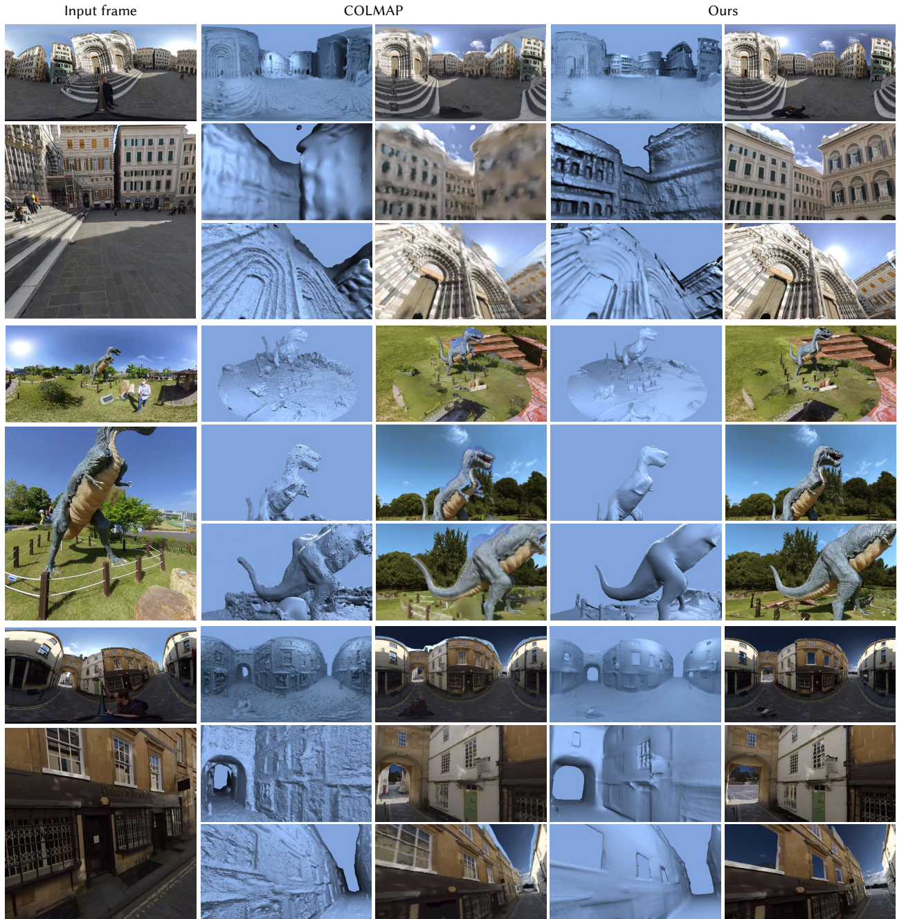
Fig. 10. Comparison of our 3D reconstruction to COLMAP [Schönberger and Frahm 2016; Schönberger et al. 2016]. Left: Input frame as spherical image (top) and perspective crop (bottom). Center: COLMAP’s reconstructed mesh and textured mesh. Right: Our reconstructed and textured mesh. The top and bottom input videos are from Bertel et al. [2020]. See our supplemental video and document for additional results and comparisons.
