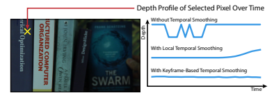
Figure 7. Our keyframe-based smoothing produces more consistent depth than local smoothing of adjacent frames. (The pixel should have constant depth in this scene.)
