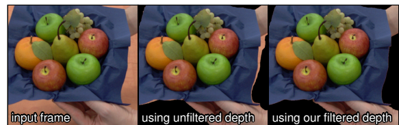
Figure 12: Examples of our video background segmentation. Our filtered depth produces clean object outlines.
